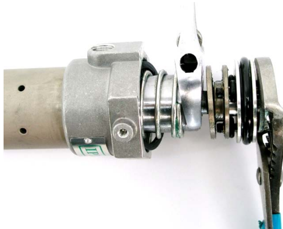
Air piston assembly with the Air Cylinder removed.
