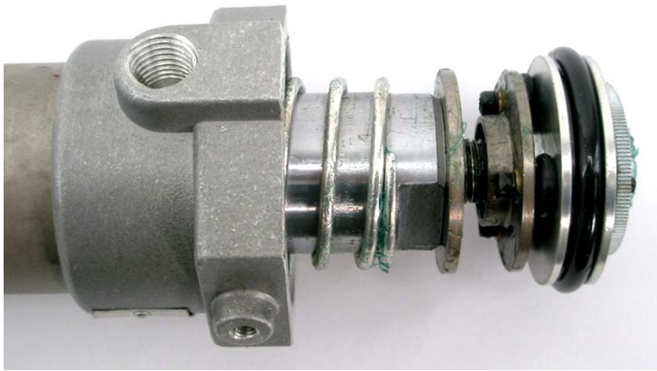
Air piston assembly with the Air Cylinder removed.
