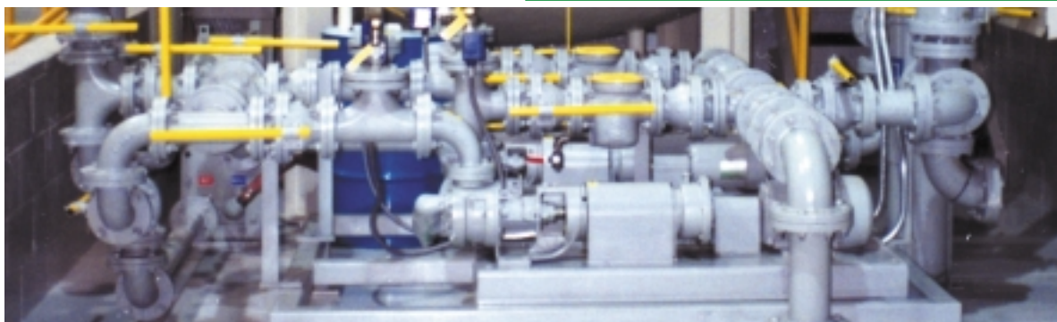
An optional two pump per component system is available with unique cross-over valving to serve as backup in case of temporary pump loss or maintenance duties. Isocyanate pumps have magnetically coupled drives to eliminate shaft seal leakage.
