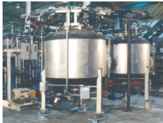
Typical Gusmer-Admiral Liquid Blending System on Load Cells.
