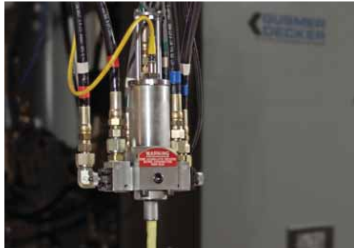
When it comes to RIM, the most critical process takes place in the mixing head. Complete mixing of the polyol and isocyanate materials is essential in order to produce quality parts.
