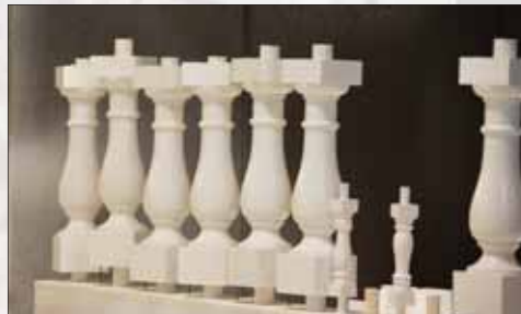
Architectural balustrades, columns, balusters, moldings and other architectural details are manufactured with the RIM process.
